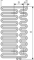
$A-Height \quad B-Width \quad C1-C5-Distance \ between \ pipe \ centres \quad D-Horizontal \ distance \ between \ mounting \ bracket \ centres \\ E-Vertical \ distance \ between \ mounting \ brackets \quad F-Distance \ between \ a \ mounting \ bracket \ and \ the \ bottom \ of \ the \ radiator$
